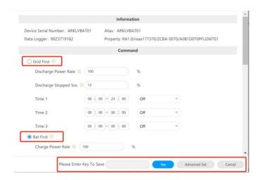
1. For Load First, it is the default setting, you can set the "Discharged Stopped SOC". The battery will stop discharging when the SOC reaches the setting value, then it will be restored after battery reaches" Discharge Stopped SOC + 3%"
